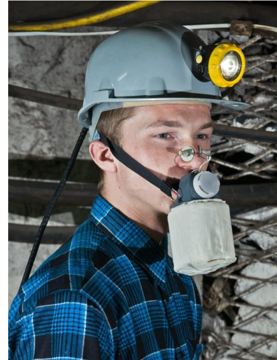
Training in the operation and use of the canister is carried out using the TPG-8 training mining canister
